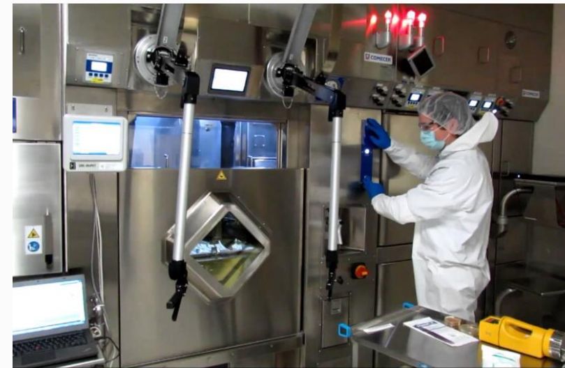
Shielded fume hood (hot cell) for radiopharmaceuticals production
