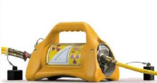
Industrial Radiography with sealed source
